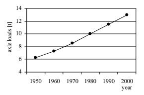
Fig. 2 Development of axle loads on German highways [1]
