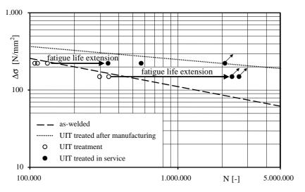
Fig. 9 Results of fatigue tests
